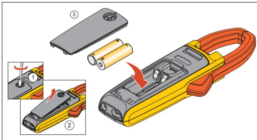
**Figure 5. Battery Replacement**
