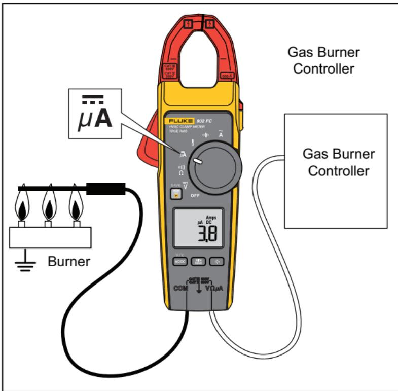
**Figure 2. Test a Flame Rod**
