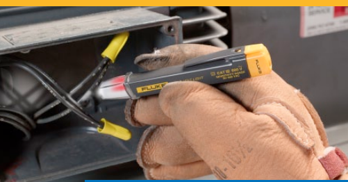
IVD2, with flashlight and dual sensitivity
