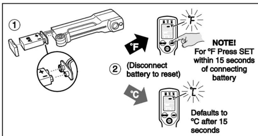
**Figure 12. Setting/Changing °C and °F Temperature Scales**
