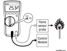
To measure flame rectification circuits:
